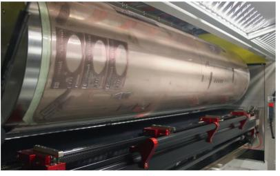
the last printing unit, a long, double-vacuum transport section has been added, with a special vacuum system to prevent dust from damaging print quality.
