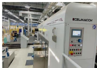
the new Chroma Print offers high performance, both in terms of quality and operation. Printing precision is ensured by direct motor technology thanks to an independent motor on each shaft.
