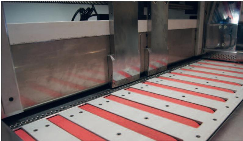
**Belt feeder is driven by independent Siemens motors.**
